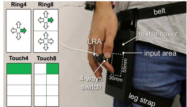
Figure 1. Ring hardware prototype and experimental setup.
